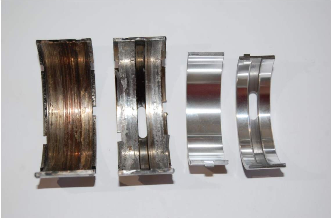
Kuva 13. Damaged crankshaft main bearings (left) and the intact main bearings (right).
